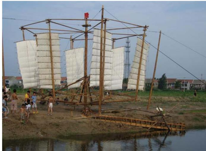
**Fig. 2.** The field-test of the vertical shaft type wind-power Chinese square-pallet chain-pump in Haihe in the northern Jiangsu province
