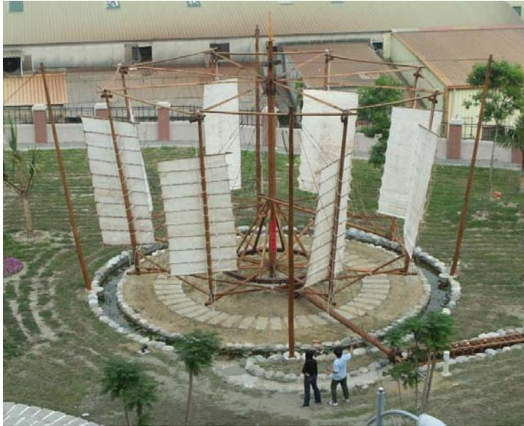
**Fig. 3.** The vertical shaft type wind-power Chinese square-pallet chain-pump stands on the campus of the Southern Taiwan University
